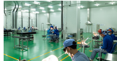
Pyro-processing of quartz by veteran engineers
