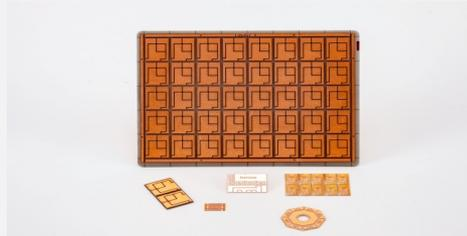
\*In response to **the global trend of power consumption reduction**, the demand from clients needing power semiconductors is growing. (DIRECT COPPER BONDING technology for bonding a copper circuit to an aluminum ceramics substrate)
